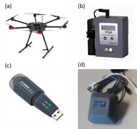
Figure 2-2 Pictures of (a) DJI Matrice 600 Pro, (b) Personal Ozone Monitoring (POM), (c) Portable Temperature and Humidity Data Logger OM-141, (d) MINIMA from Applied Particle Technology.
