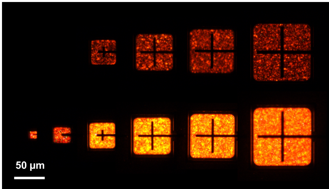
Figure 4.15: Microscope images of electroluminescence of red microLEDs at 1 and 10 \text{A}/\text{cm}^2
