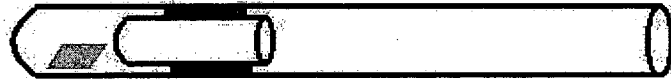
Figure 2-9: Schematic of sealed ampoule with gray semiconductor diffusion sample sealed in small volume.
