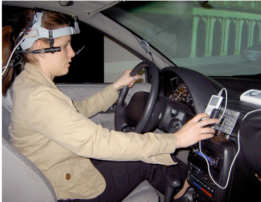
Figure 12: The 20 GB iPod shuffle mounted on the center console in the simulator
