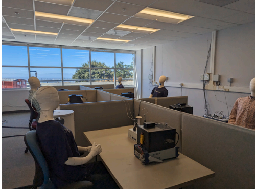
Fig. 1. Layout of the FLEXLAB test cell. It is configured as an office room in this experimental demonstration.
