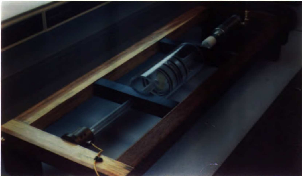
Figure 14: Perspective view of the second compression device that was designed to apply step loads rather than step displacements. The non-magnetic stainless steel pneumatic cylinder (upper right) was pressurized with nitrogen gas to apply the loads. The force transducer (lower left) allowed recording the actual loads applied while scanning.
