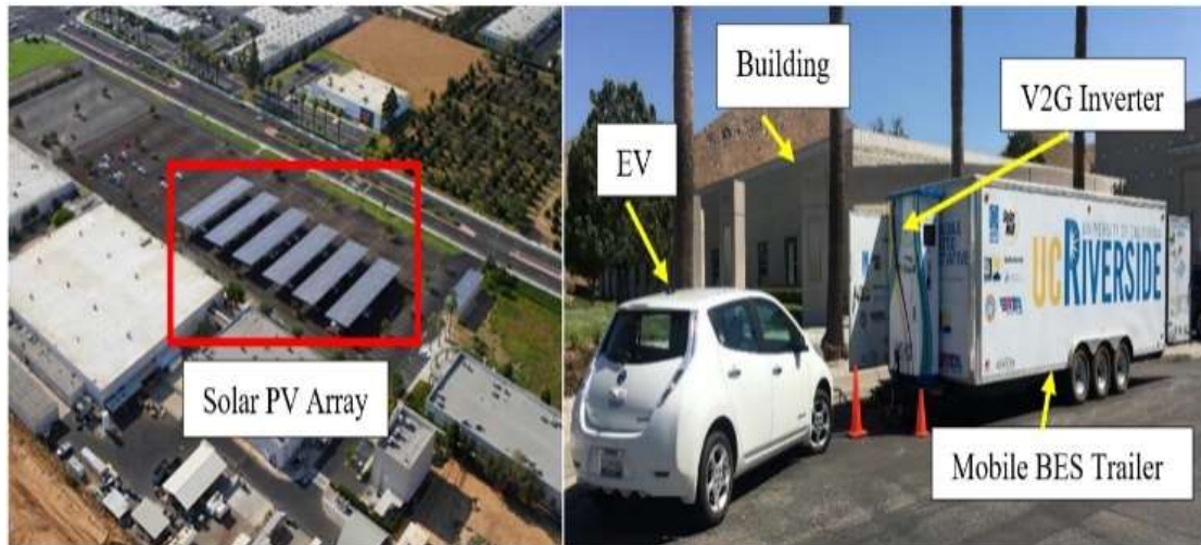
Figure 5-1 Different components of the microgrid
