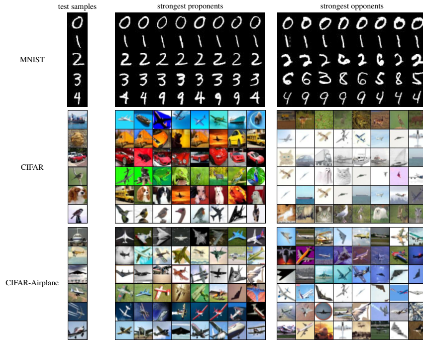
Figure 3.4. Test samples, their strongest proponents, and strongest opponents. In MNIST the strongest proponents are visually similar while the strongest opponents are often the same digit but are visually different. In CIFAR and CIFAR-Airplane the strongest proponents have similar but brighter colors.
