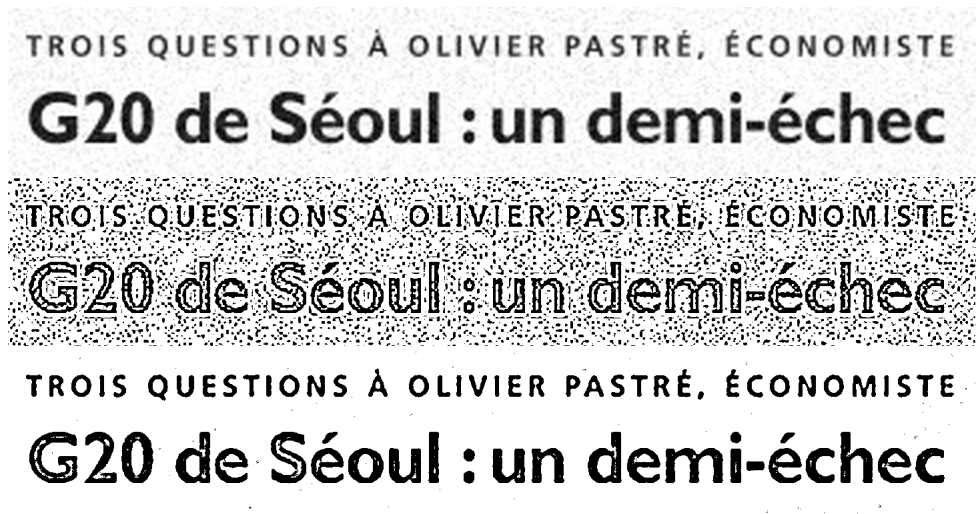
Figure 3.7: Top: Noisy grayscale GP upsampled text block. Middle: Adaptive thresholding with no filter. Bottom: GP upsampled image with bilateral filter and adaptive thresholding.
