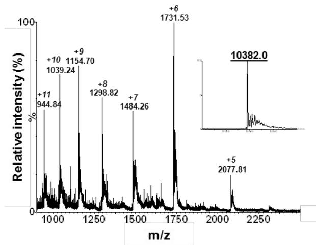
**Figure 2.** ESI mass spectrum showing the charge state distribution of ELP20. Charge states of the highest intensities are labeled with their charges. Inset: MaxEnt-deconvoluted ESI mass spectrum of ELP20.
