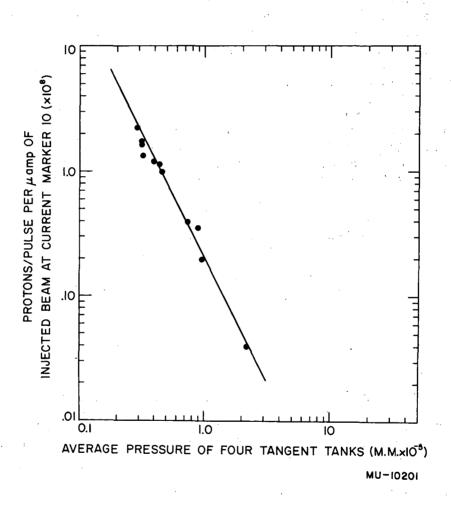
Fig. 4. Protons/pulse per  $\mu$  amp of injected beam at 100 Mev as a function of average pressure of four tangent tanks.
