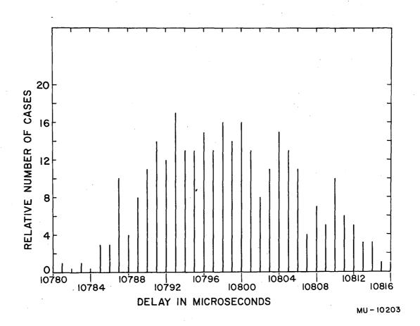
Fig. 6. Time fluctuation in microseconds between marker 3 and marker 4; 300 consecutive pulses, 4500 amps/pulse, 15 pulses/min; I - pip 3 = 110.1 amps, I - pip 4 = 139.0 amps.
