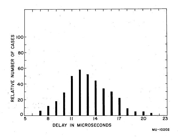
Fig. 5. Jitter in start frequency, determined by difference between time of rf turn-on signal and 1st frequency pip. Total of 377 consecutive pulses. Pulse rate 14 per minute. Magnet pulsing to 4500 amps.
