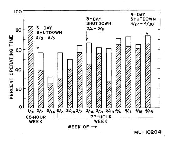
Fig. 7. Bevatron operating time. Height of bar indicates actual operating hours as a fraction of nominal operating week. The shaded portion represents time on physics research.
