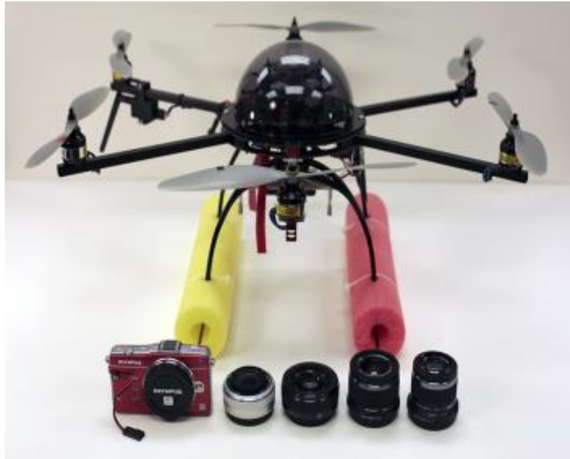
Figure 2. Image showing the APH-22 hexacopter (Aerial Imaging Solutions, Old Lyme, CT) that was used to fly 332 successful flights to collect vertical photogrammetry images of killer whales at sea. Here shown with the Olympus E-PM2 camera and interchangeable lens system; the camera mounts on the underside of the hexacopter to be downward-facing (Durban et al. , 2015).
