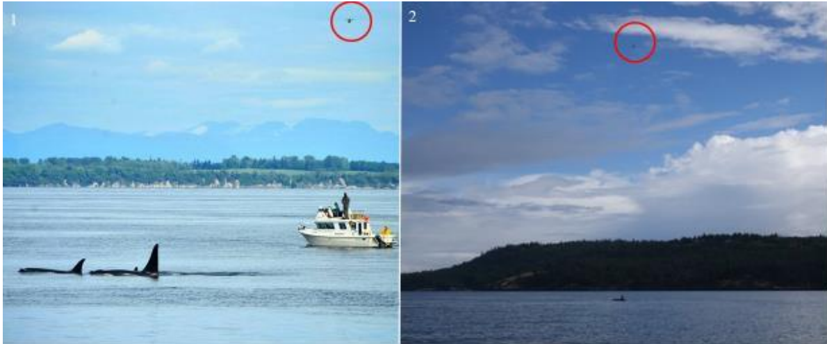
Figure 4. 1) Image showing the hexacopter (circled) being deployed from the upper deck of a 8.2 m research vessel. 2) Images showing the hexacopter capturing vertical images of killer whales from an altitude of > 30\text{m} .
