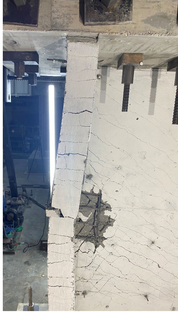
Figure 6-7: Damage state of the east flange after the completion of testing, CW-3
