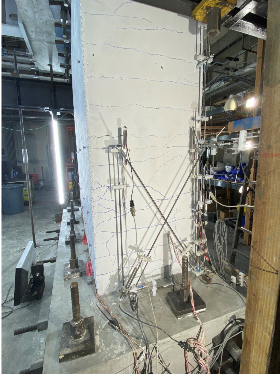
Figure 3-8: Cracking condition of CW-1 at the end of WLP (Outside surface of the East flange)
