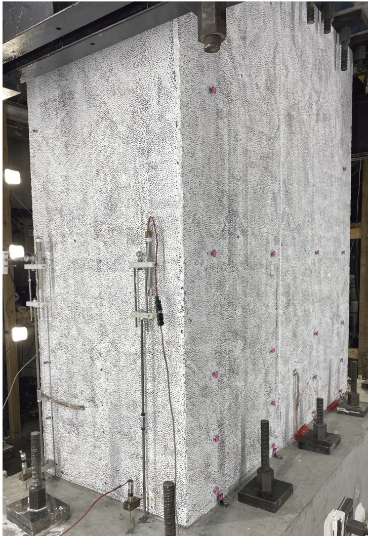
Figure 2-33: Digital image correlation pattern
