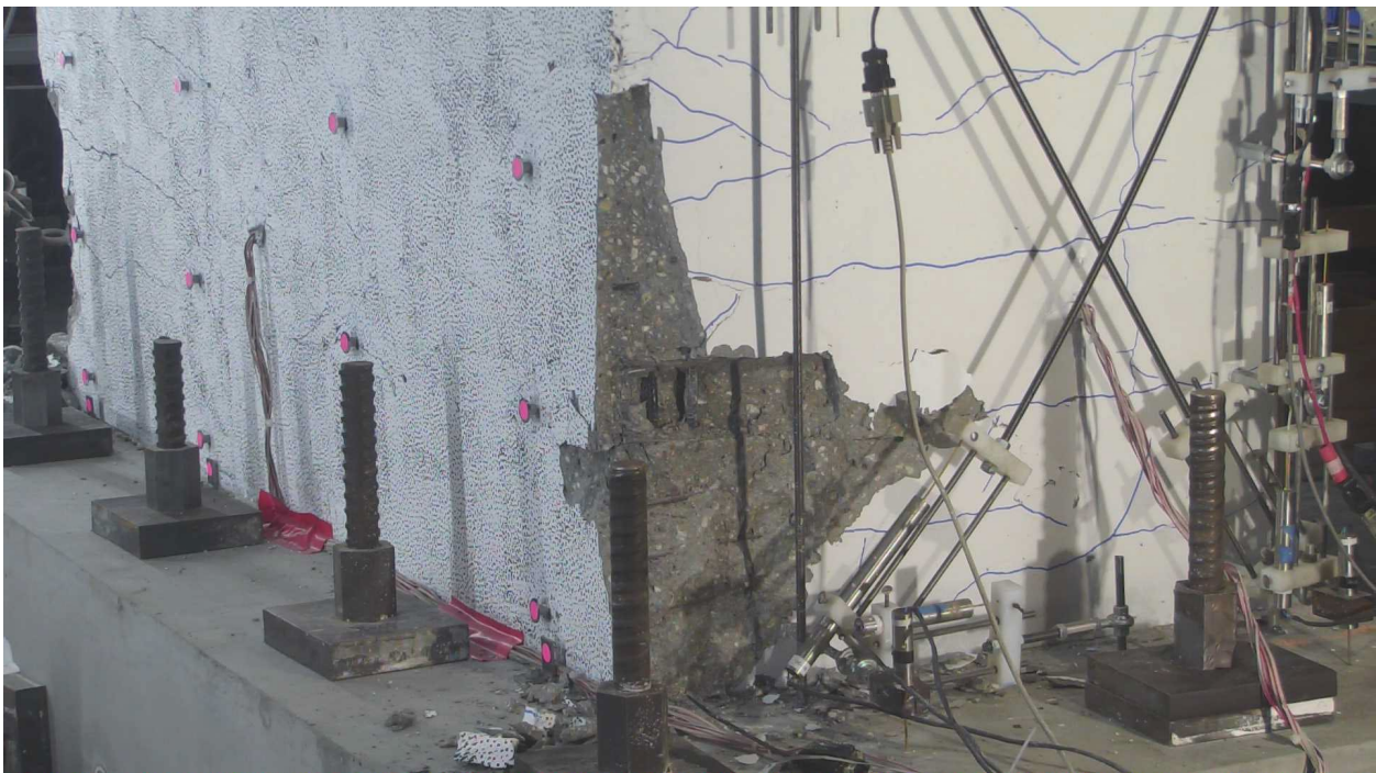
Figure 4-4: Damage state of the East flange and the web after the first cycle at 2.0% hinge rotation demands (at zero loads)
