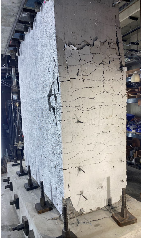
Figure 6-7: Damage state of the east flange after the completion of testing, CW-3
