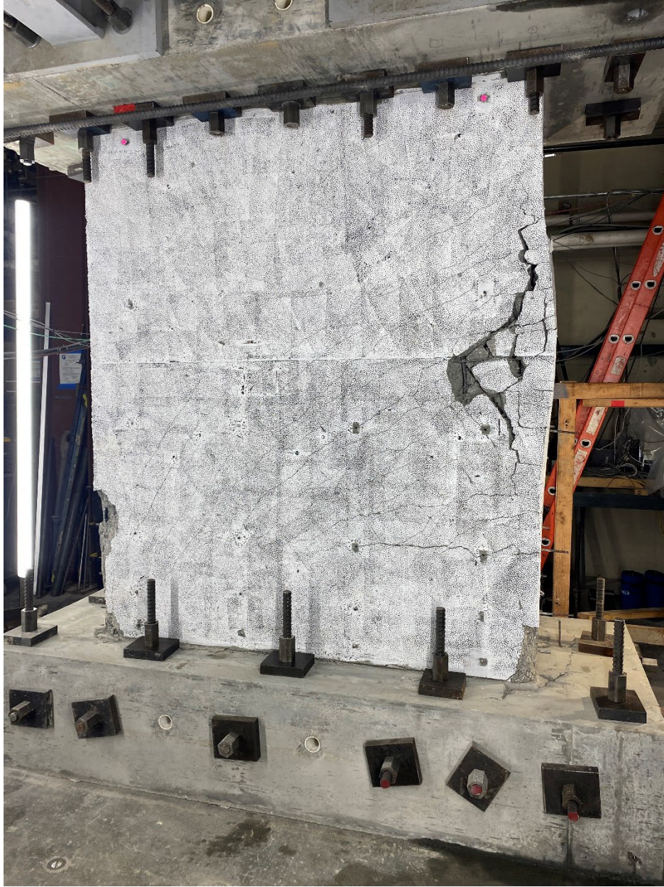
Figure 6-8: Damage state of the web after the completion of testing, CW-3
