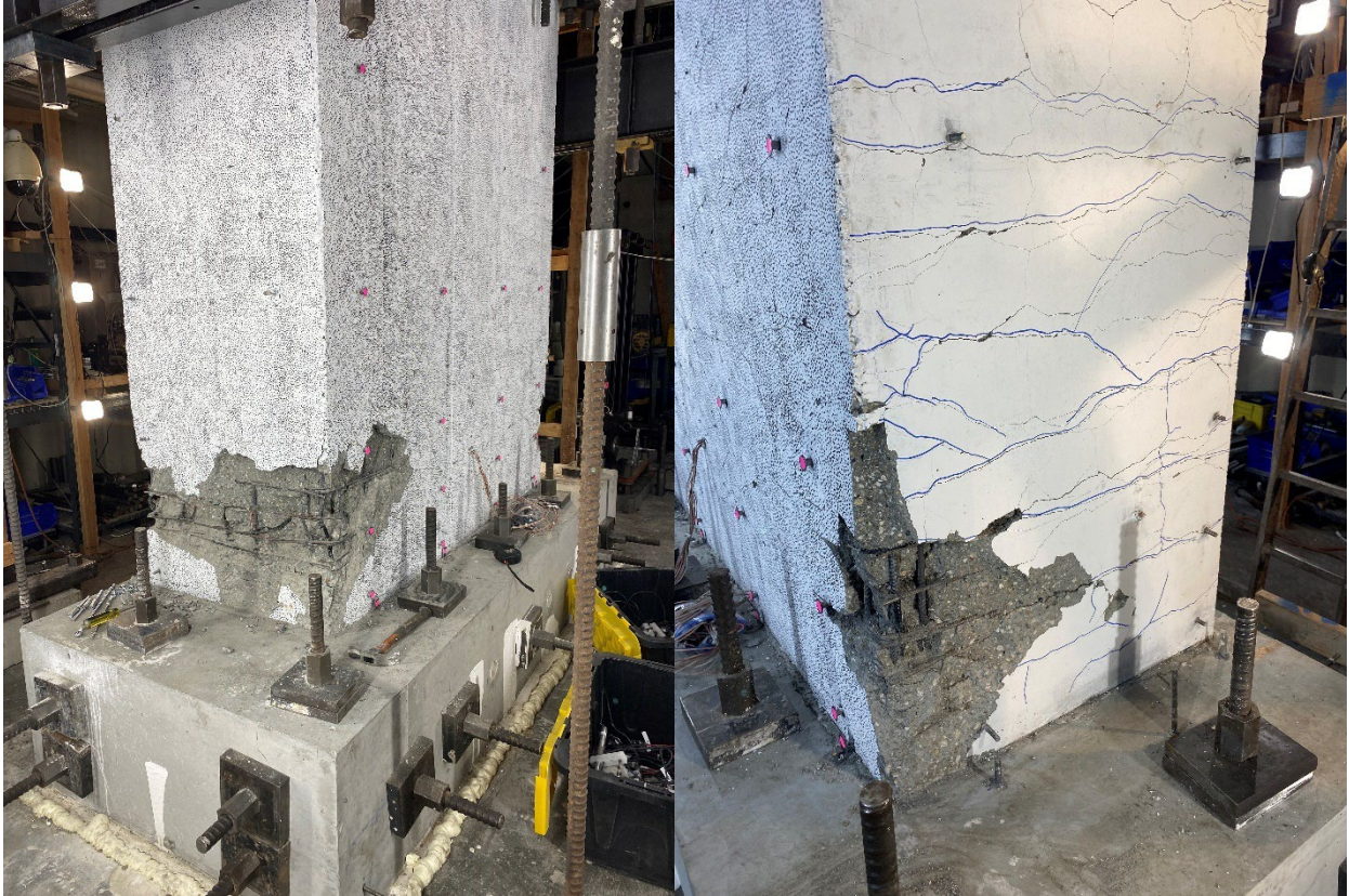
Figure 4-5: Damage state of the West flange (left) and the East flange (right) after the test
