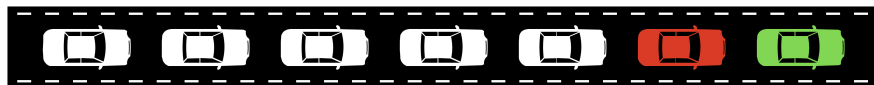
Figure 7.4: Vehicle formation used in simulation. A trajectory leader (in green) driving a speed profile drawn from the dataset is placed in front of an AV (in red) which is followed by a platoon of 5 human vehicles (in white), modeled using the Intelligent Driver Model.
