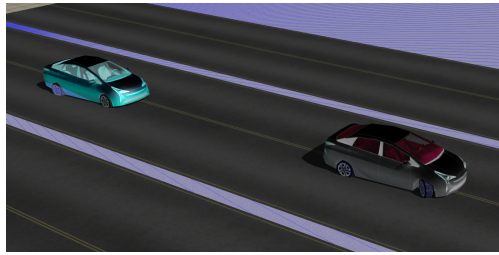
Figure 7.5: The 2-vehicle simulated scenario used for assessing the behavior of the RL controller. The lead car performs a series of abrupt starts and stops that the RL car behind it must safely respond to.
