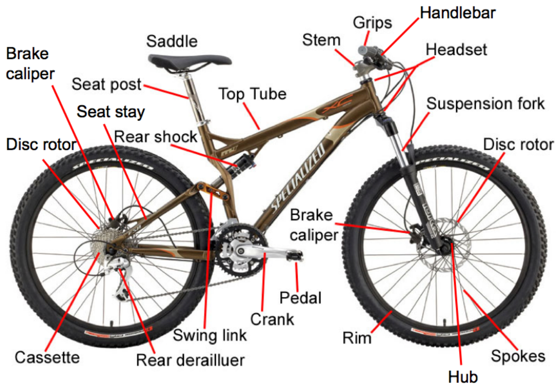
Figure A.1: Diagram of the majors parts of a full suspension bicycle. [4]
