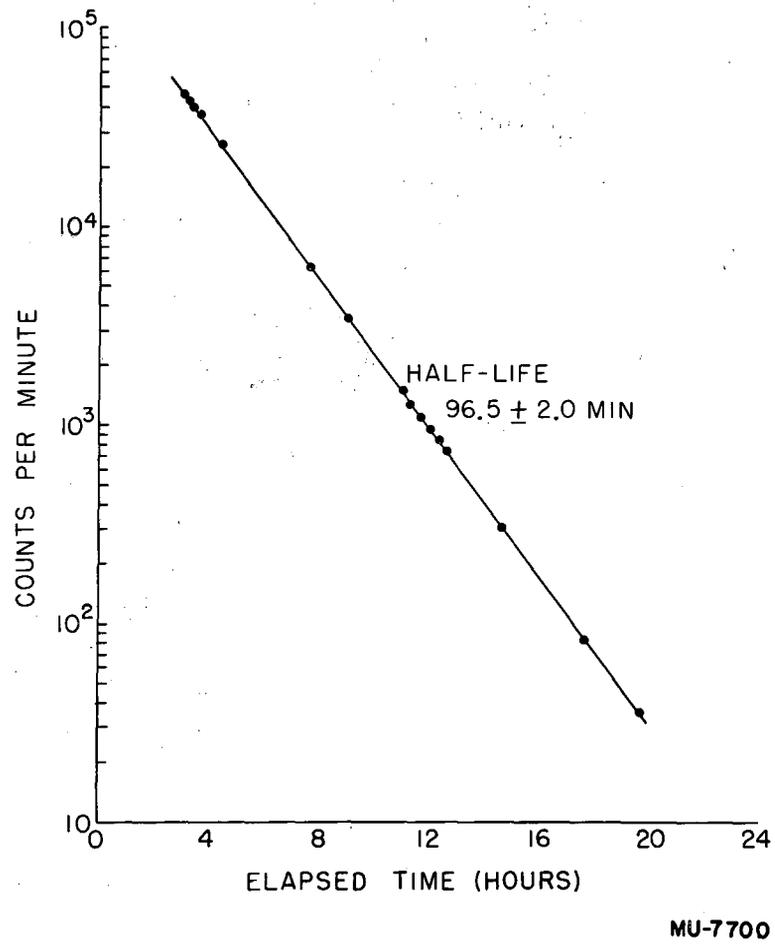
Fig. 1. Geiger-counter decay curve of Ba126.
