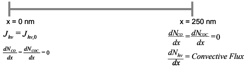
Figure 7.2 One-dimensional, numerical model developed in COMSOL TM to simulate VUV photon penetration depth and C = O density profiles. The PR surface is defined x = 0 and receives a photon flux: J_{hv,0} .
