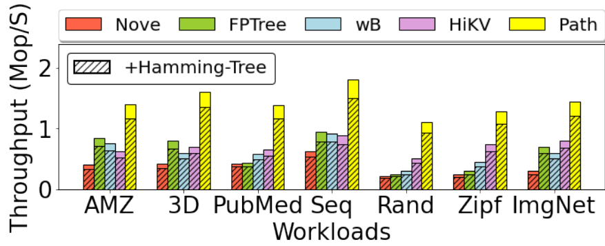
Figure 5.16: Throughput of different methods before and after being augmented by Hamming Tree.
