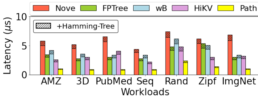
Figure 5.15: Write latency of different methods before and after being augmented by Hamming Tree.
