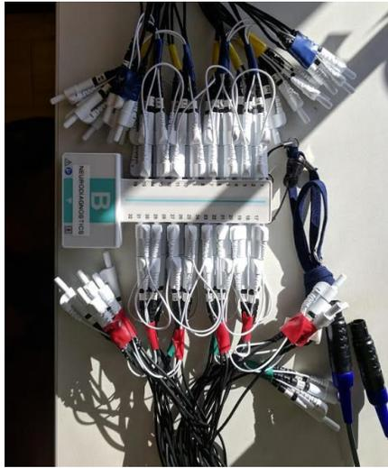
**Figure 2.7:** Touch proof jumpers are used to short/ connect the
