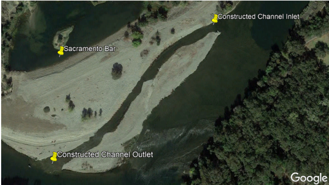
Figure C: Side channel constructed in 2016 at Sacramento Bar that was flooded out in January of 2017. The constructed channel inlet and outlet are shown.
