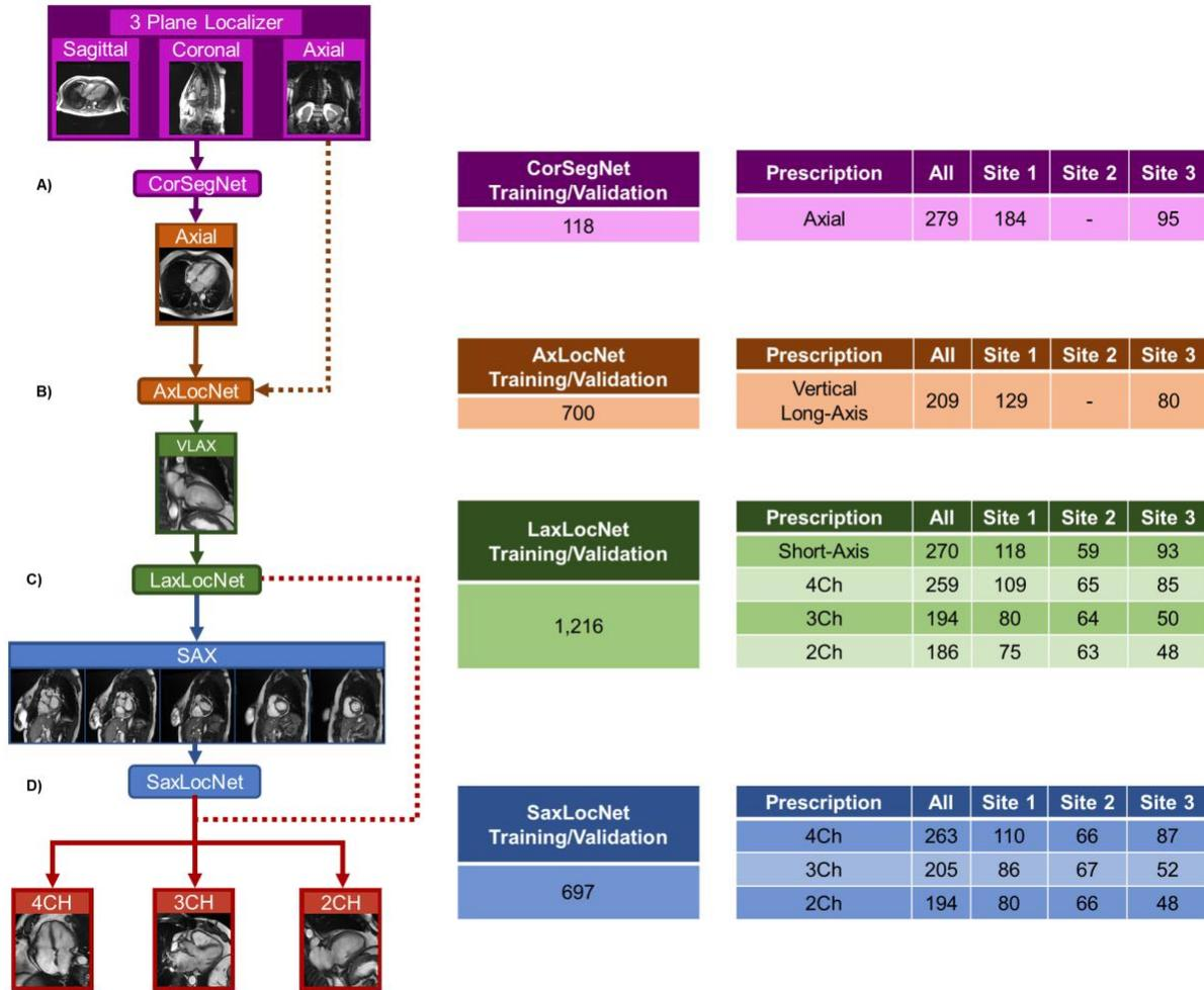
**Figure 7:** Left) Schematic of an automated, multi-stage system for prescribing cardiac imaging planes comprised of multiple DCNN modules and Right) number of image series used for either training/validation or testing.
