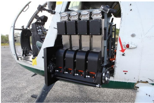
Figure 2. Automated dispensing module (ADM) comprised of four magazines carrying 900 bait cartridges each. Mounted in Wildlife Services Hughes OH-6 helicopter.
