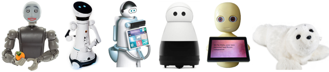
Figure 2.1. Robots used to support people with cognitive impairments vary widely in morphology, including mobile, tabletop, humanoid, mechanistic, and zoomorphic. From left to right: Bandit [439] (Provided by Maja Matarić), Care-O-bot [243] (Provided by Fraunhofer IPA [139]), KOMPAĚ-2 [12] (Provided by KOMPAĚ Robotics [245]), Kuri [256] (Provided by Mayfield Robotics), Mabu [84] (Provided by Catalia Health), PARO [474] (Provided by Carlton SooHoo [339]).
