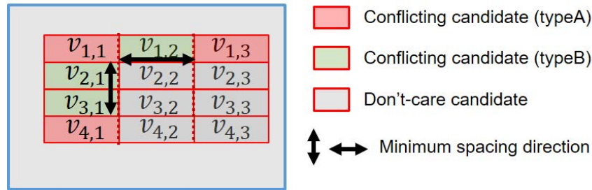
Figure 2.26: Illustration of conflict list enumeration for minimum spacing constraint, showing horizontally and vertically conflicting pairs.
