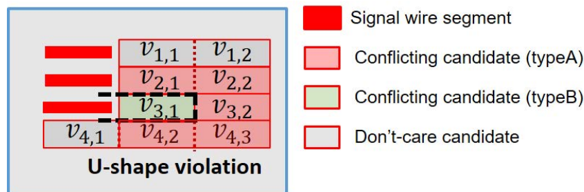
Figure 2.21: Illustration of a U-shape block mask rule violation.
