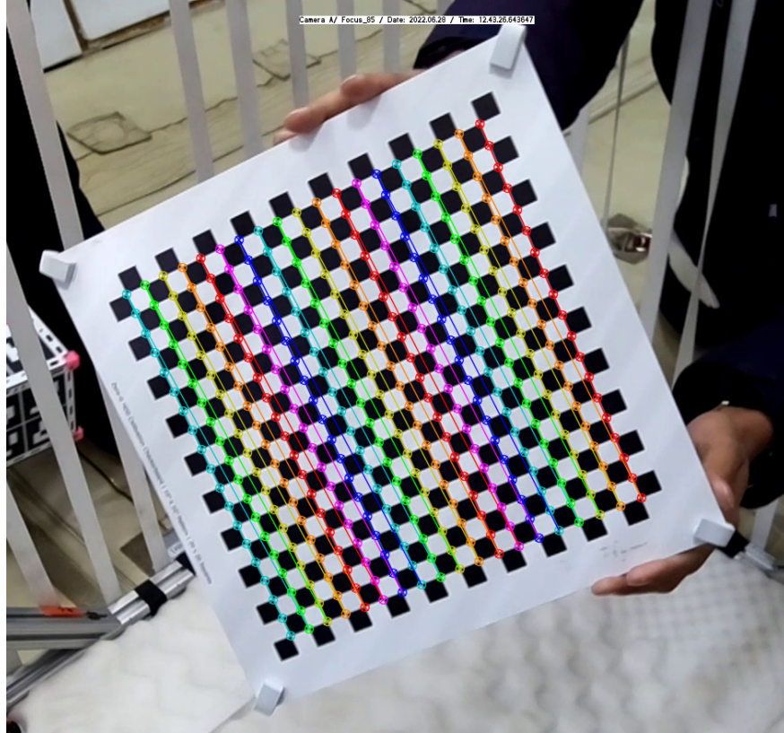
Figure 3.7: Calibration target with checkerboard corners detected (indicated with colored circles) and rows detected (indicated with straight lines connecting like-colored circles)
