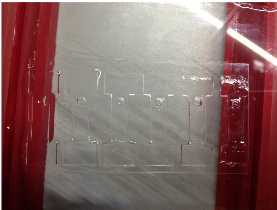
Figure 4-24: Photograph of photopatterned polyacrylamide free-standing gel for use with IEF.
