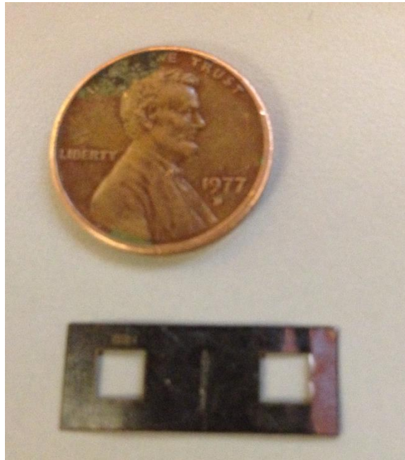
Figure 4-8: Laser cut steel mask (fabricated by Rob Lin) used for UV photopatterning. Small slit in center used for patterning and larger squares are for alignment on the wells.
