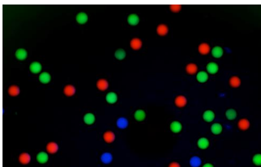
Figure 3-5: PEG-diacrylate beads spectrally encoded with lanthanide nanoparticles. (Image generated by Kurt Thorn)
