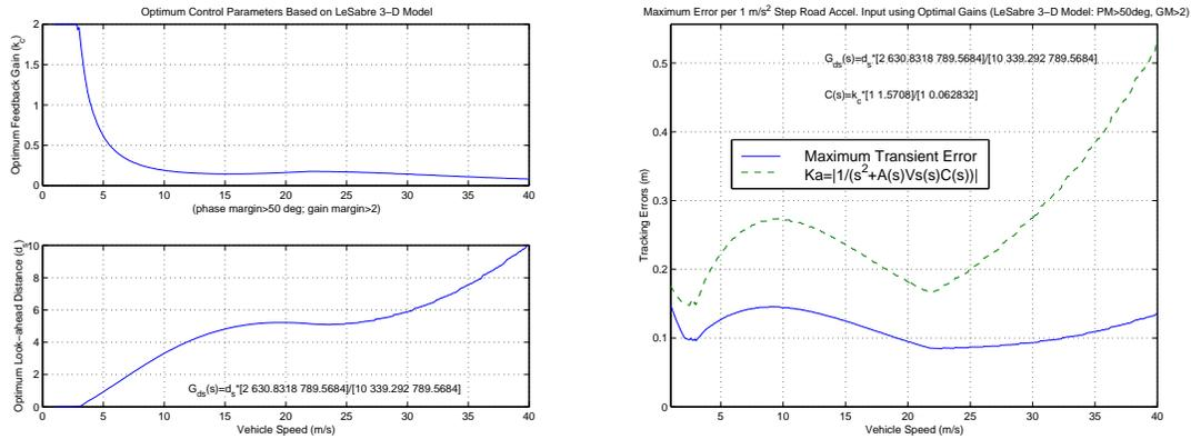
Fig. 5. Optimal control gain pair  $(\bar{k}_c, \bar{d}_s)$  and resultant maximum transient error based on 3 DOF model with frequency shaped look-ahead control ( $pm=50$  deg,  $gm=2$ )
