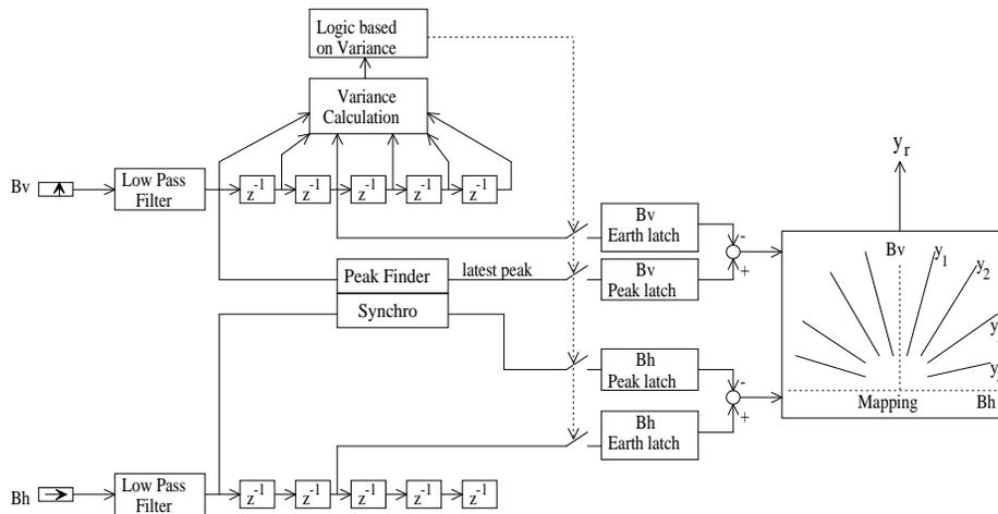
Figure 3.2 “Peak-Mapping” Magnetometer Signal Processing Block Diagram
