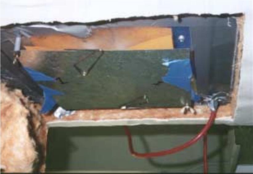
**Figure 6. Impaction plate installed in Building LS-2**
