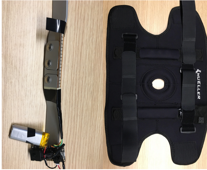
Figure 4.4: The system before placing on the knee brace (left) and the final version of the system in the knee brace (right).
