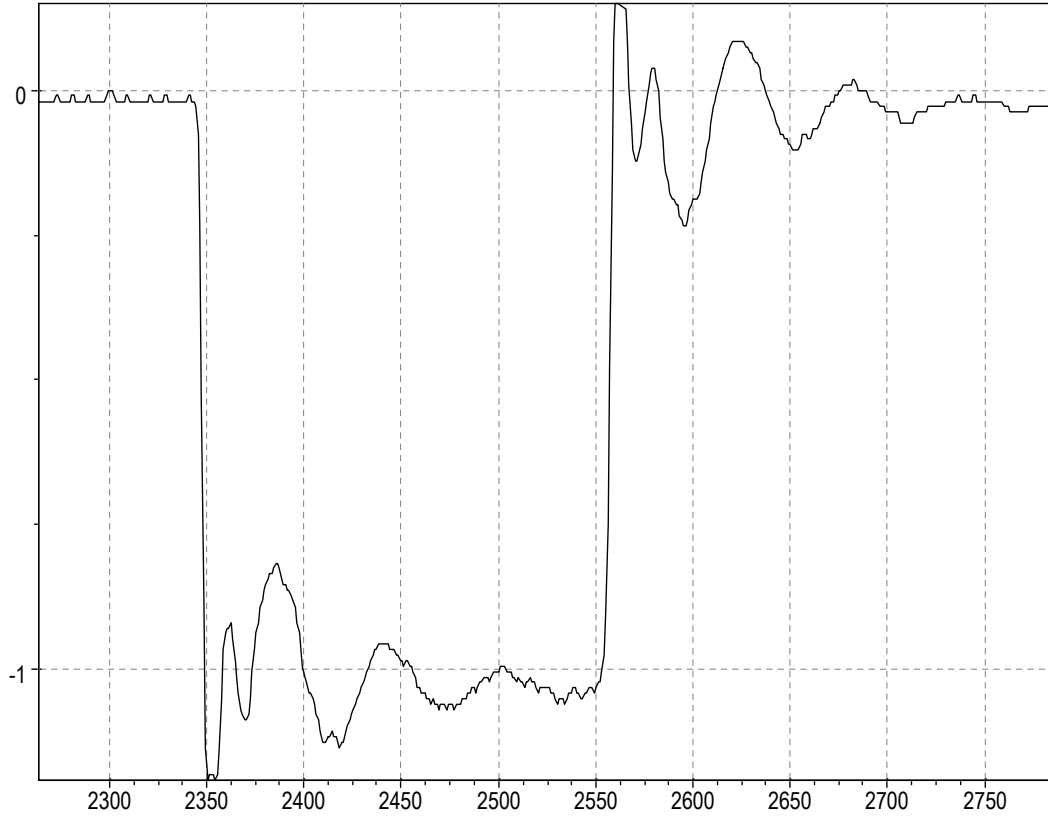
Figure 4.3: Oscilloscope trace of pulsed gate voltage V_g for original (Janis factory) cryostat sample insert. After switching on, ( t = 2350 ), considerable ringing and voltage overshoot due to impedance mismatch is evident. The ringing has barely damped even \sim 150 ns later when V_g is switched off, and new ringing and overshoot are again induced. The impedance mismatch slows the transition edge (ie, reduces the rise/fall times), and the ringing causes the indirect excitons to oscillate in energy. Vertical scale in volts.
