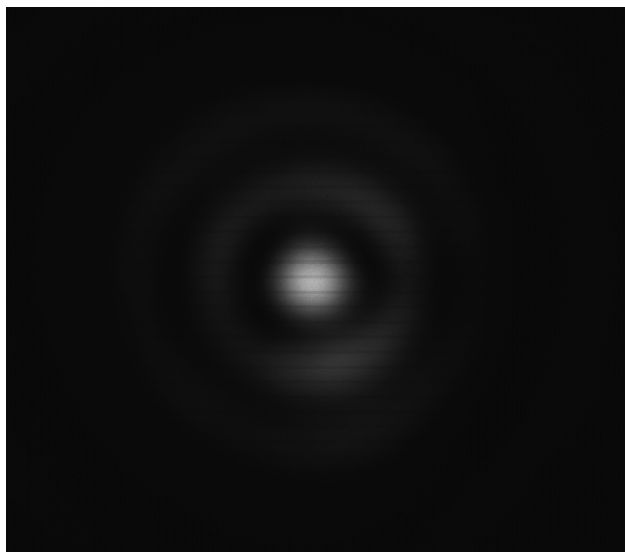
Figure 2.17: A typical profile of the optical (pump) beam taken by the CMOS camera (Fig. 2.16). The rings are due to beam diffraction on the annular mirror.
