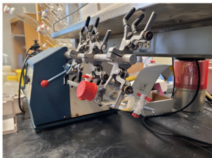
Fig. 6 (A) SPPS flow chart of compound 13; (B) resin swelling, 1st amino acid loading, capping, and cleavage are performed by shaking; (C) amide coupling and Fmoc removal reaction are stirred by bubbling; (D) liquid phase is pushed out of the SPPS vessel with air or nitrogen to separate it from beads.
