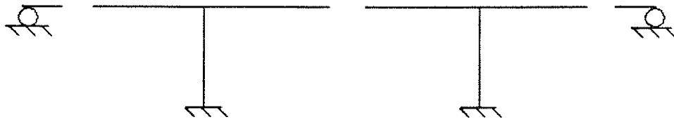
A) INITIAL STRUCTURAL SYSTEM (CANTILEVER)
