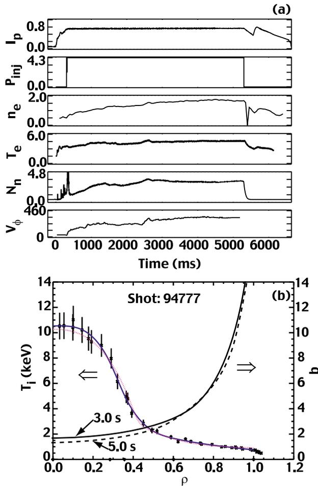
FIG. 4 (color online). Plasma characteristics for shot 94777: (a) Plasma current  $I_p$  (MA), injected neutral beam power  $P_{inj}$  (MW), line-averaged electron density  $n_e$  ( $10^{19} \text{ m}^{-3}$ ), core electron temperature  $T_e$  (keV), total neutron emission rate  $N_n$  ( $10^{14}$  neutrons/s), and core toroidal rotation velocity  $v_\phi$  (km/s). (b) Ion temperature profile and  $q$  profile at  $t = 3.0$  and  $5.0$  s.
