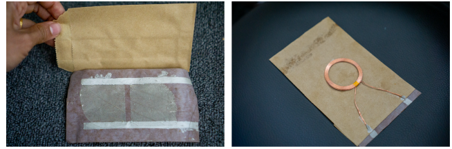
Figure 5: Left: Open-faced view of the leaves, silver traces, and paper packaging. Right: Reverse side of packaging showing charging coil (off-the-shelf copper coil used as stand-in for printed silver coil).
