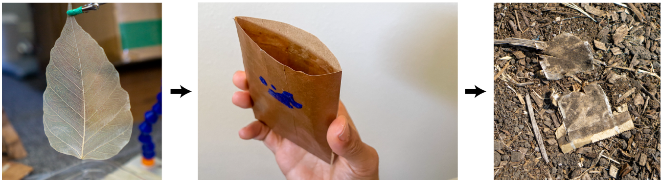
Figure 1: From leaf skeletons (left), we create a lightweight packaging that can wirelessly heat its contents (center) and is fully backyard-degradable (right).
