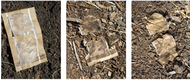
Figure 10: Left: packaging before being buried in soil on day 1. Middle: packaging dug up after 15 days. Right: packaging dug up after 30 days.
