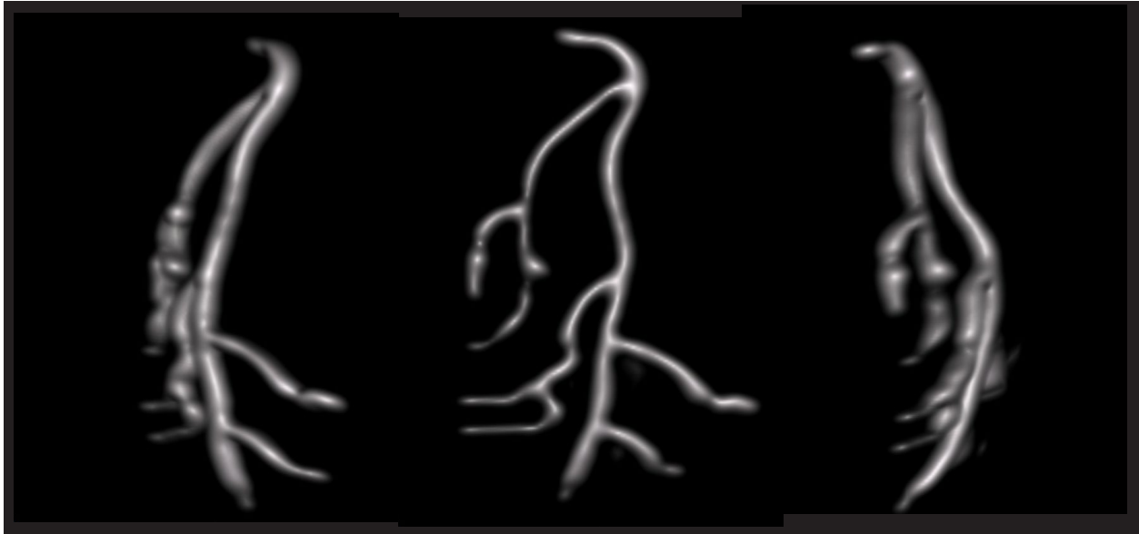
Figure 5.7: Experimental data of a coronary artery phantom from Fig. 5.6 at different angles. The 3D volume-rendered datasets were reconstructed using the proposed method with deconvolution. The total imaging time was 10 min with a field of view of 4.5 cm by 3.5 cm by 9.5 cm ( x,y,z ).
