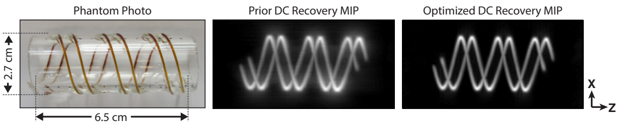
Figure 5.4: Experimental MPI data from a double helix phantom. The 3D dataset was reconstructed using the previous DC recovery method and the proposed method. Both datasets are shown in maximum intensity projection images with no deconvolution. Images reconstructed with the proposed method contain less background haze and fewer artifacts. The imaging phantom was constructed by wrapping two 0.6 mm ID tubes injected with Micromod Nanomag MIP MNPs around an acrylic cylinder of OD 2.7 cm. The total imaging time was 10 min with a field of view of 4.5 cm by 3.5 cm by 7.5 cm (x, y, z) .
