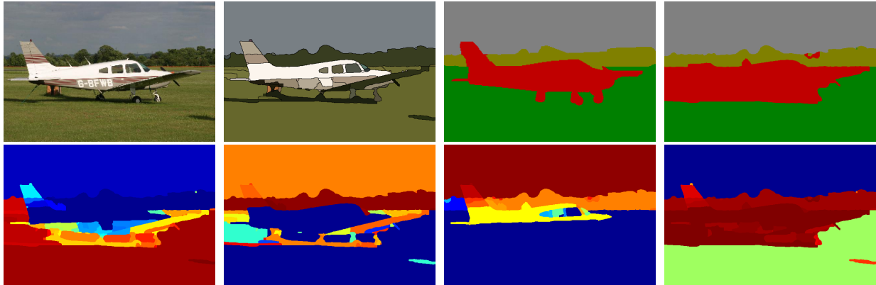
Figure 3.3: Example of merging the per category confidence maps into a single segmentation. Top: Original image, initial partition, ground truth and final segmentation. Bottom: Confidence maps for the categories grass, tree, sky and aeroplane. The confidence maps of all the categories are used to produce the final segmentation.
