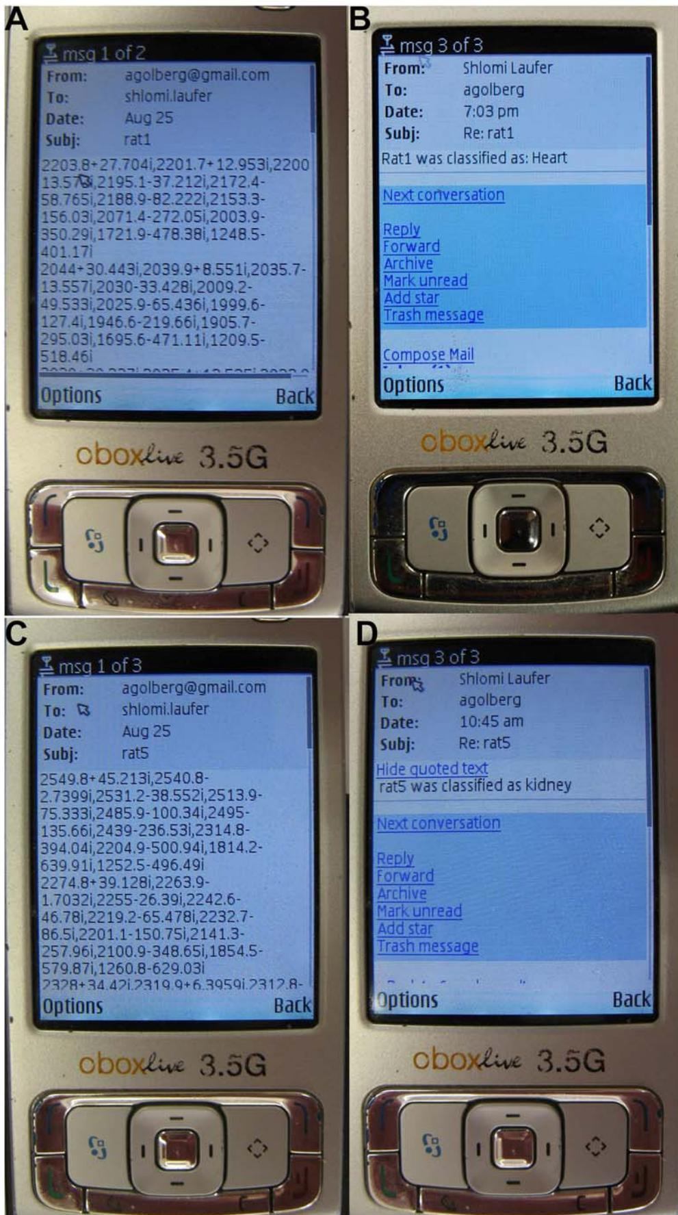
**Figure 4. Implementation of classifier using the cellular phone.** a) Measured rat heart data sent; b) Heart result received; c) Measured rat kidney data sent; and d) Kidney result received.
