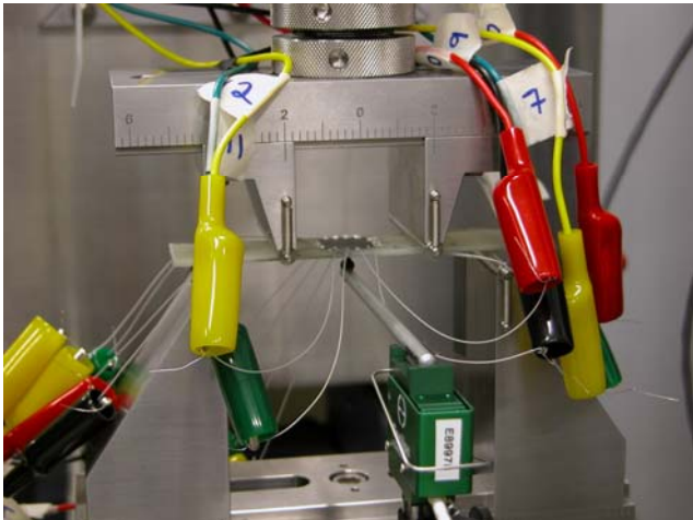
Fig. 5 Four-point bending specimen in flexure fixture.
