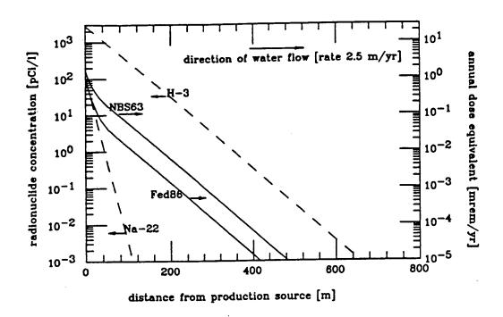
In Figure 1 the initial condition for 1 mrem/yr is based on FED86, which is used in the CEBAF design.
