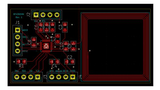
Figure 3.1: NFC Device PCB
