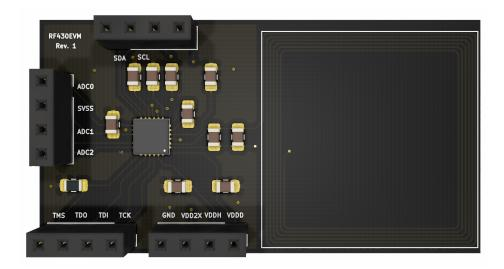
Figure 3.4: NFC Device 3D Model
