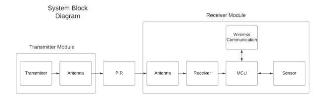
Figure 2.1: System Block Diagram
