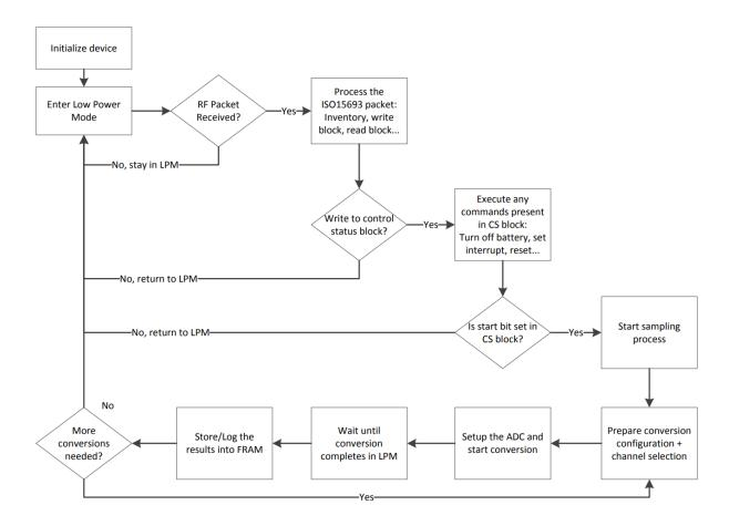
Figure 3.6: RF430 Firmware Flow
