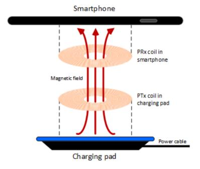
Figure 1.2: Qi Wireless Power Transfer [7]
