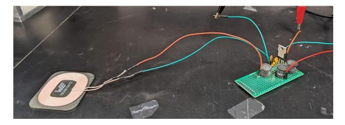
Figure 3.10: Class E Amplifier on Protoboard
