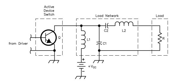
Figure 3.8: Class E Amplifier Schematic
