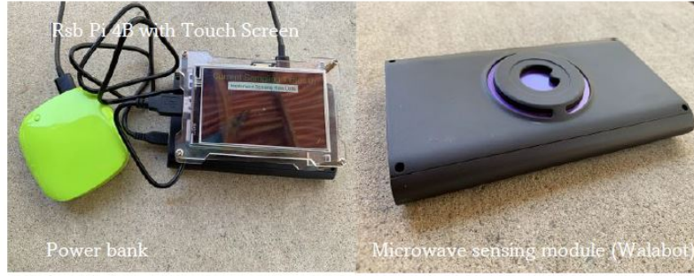
Figure 3.1: System hardware, left is the Raspberry Pi 4B with visualization user interface, and right is the Walabot microwave transmitter and receivers.
