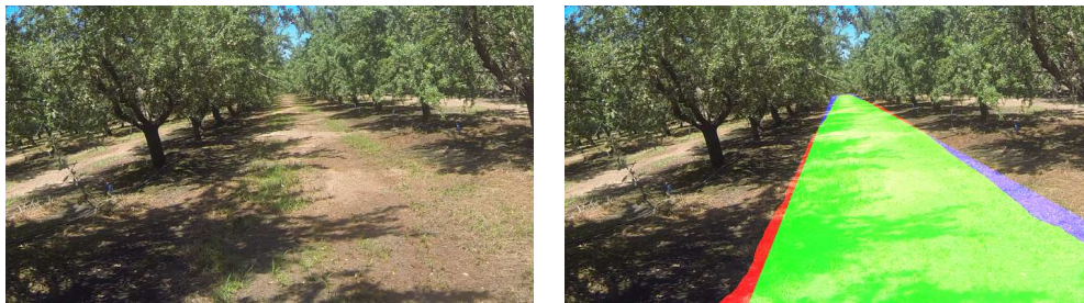
Figure 2.32: Field road recognition, green color indicates true positive, red indicates false positive, and purple represents false negative.
