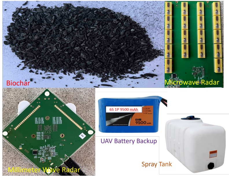
Figure 4.11: The payload options of the mobile platforms. The biochar, microwave radar, millimeter wave radar, battery, and spray tank are shown individually.
