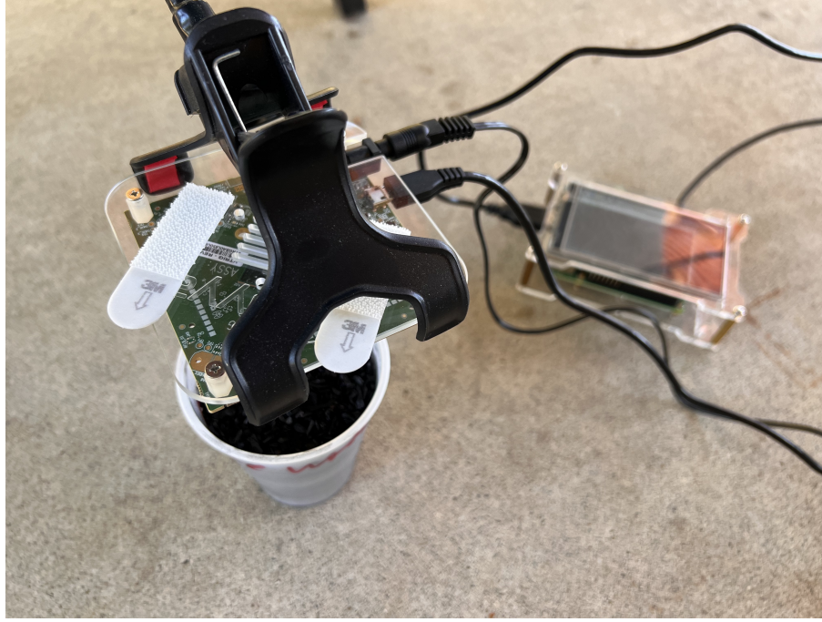
Figure 3.2: Millimeter wave radar sensor with Raspberry Pi Setup.
