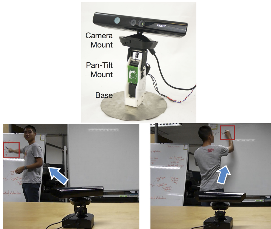
Figure 7.1: Kinectograph includes a Kinect camera to track user movement and a motorized dock to pan and tilt the camera so that the user (or their hand) remains centered in the recorded video. Here the device follows the user’s hand while he is illustrating.
