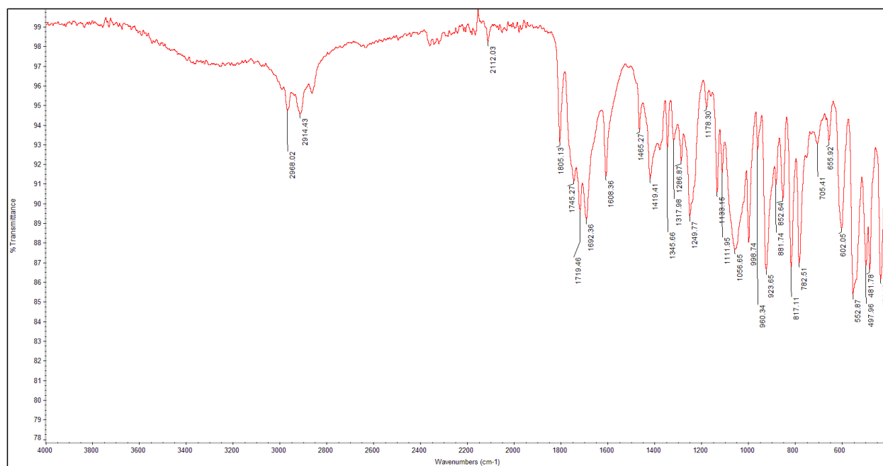
Figure 3.9. ATR-IR spectrum of a sample of single crystalline Ni(TIB Mes 2H) 4 after 2 minutes of air exposure. Free TIB Mes 2H isocyanide is observed in the spectra at 2112 cm -1 .
