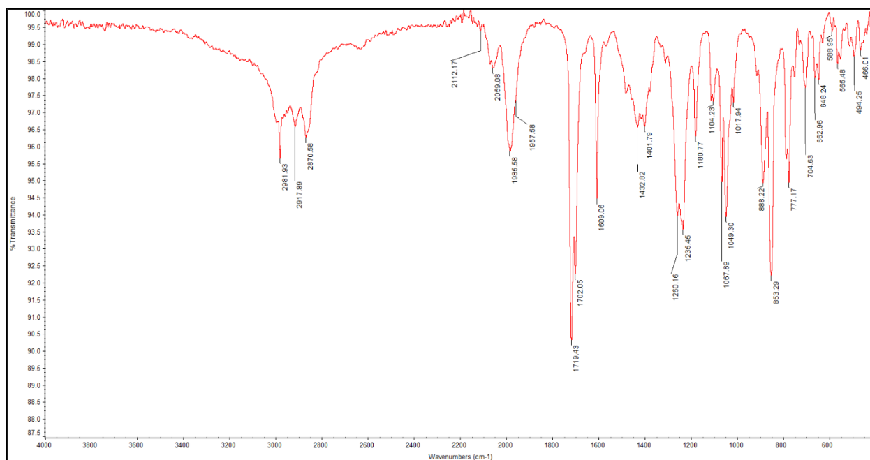
Figure 3.8. FT-IR spectrum of a THF solution containing 4 equivalents of TIB Mes 2H and 1 equivalent of Ni(PPh 3 ) 4 .
