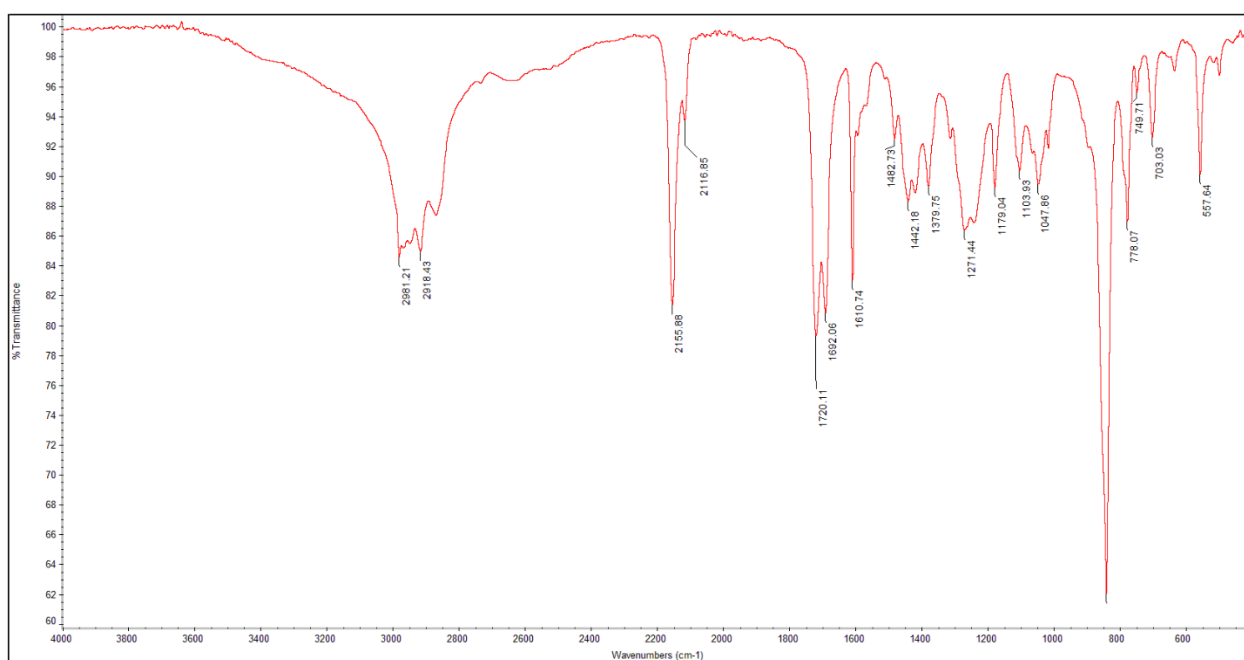
Figure 2.21. Solid State ATR-IR spectrum of 4.0 equiv TIB Mes 2 and [Cu(NCMe) 4 ]PF 6 showing presence of free TIB Mes 2 .
