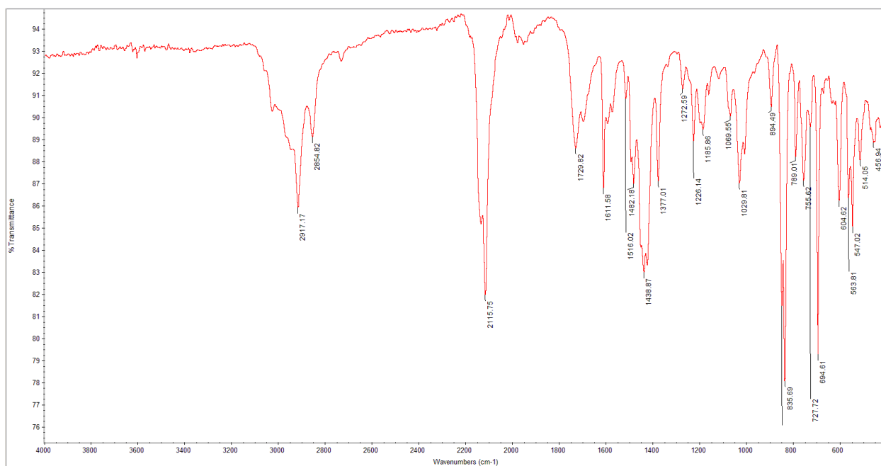
Figure 4.28. ATR-IR of a sample of Ni ISO CN-3 after treatment with 3 eqvt. BnBr at room temperature over the course of 24 hours. Decomposition of the material is observed as free ligand is the only present isocyanide stretch.
