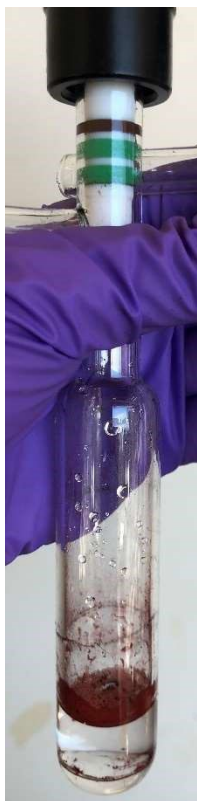
Figure 4.25. Ni- ISO CN-3 in an ampoule with 3 mL of Millipore water. The red sample floats on top and sticks to the walls of ampoule and does not mix with the water.
