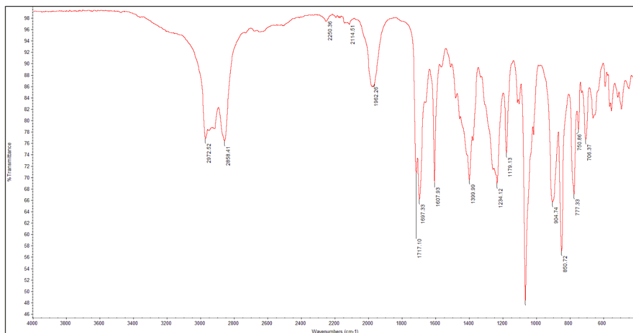
Figure 3.10. ATR-IR spectrum of a crystalline sample of \text{Ni}(\text{TIB}^{\text{Mes}2\text{H}})_4 after \text{CO}_2 gas sorption measurements were taken. The isocyanide stretching frequency at 1962\text{ cm}^{-1} indicates \text{Ni}(\text{TIB}^{\text{Mes}2\text{H}})_4 did not decompose during activation and gas sorption measurements. There is some isocyanide observed at 2250\text{ cm}^{-1} due to air exposure after measurement was taken and the sample was removed from the instrument.
