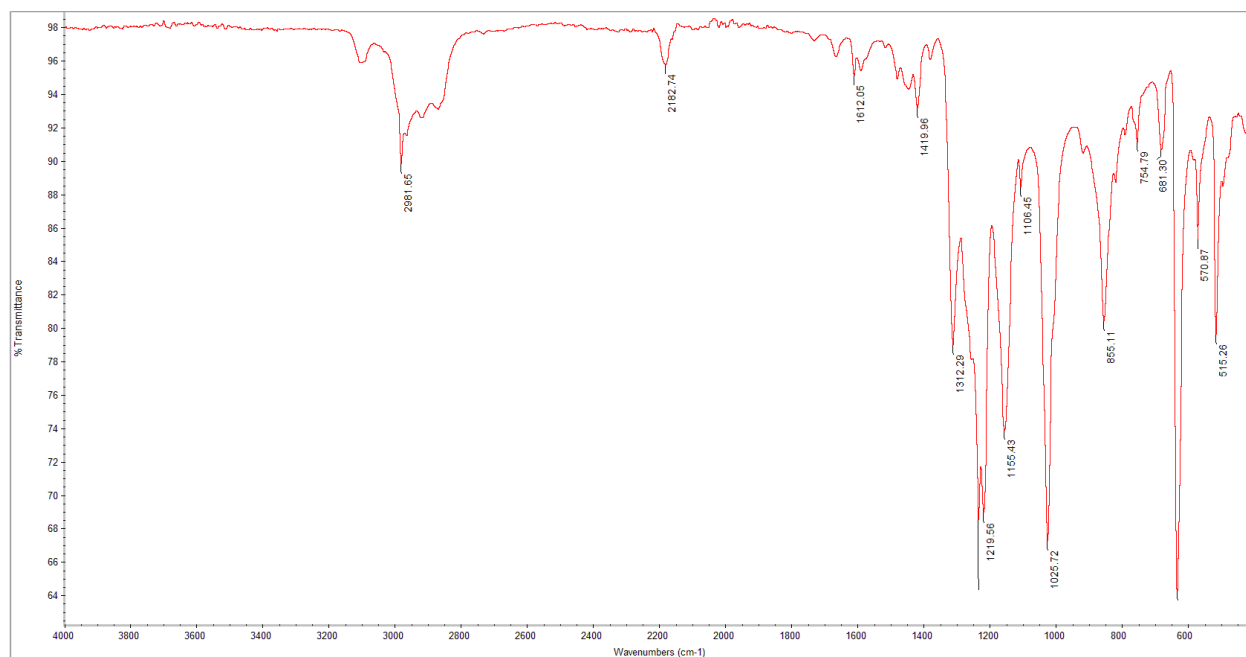
Figure 4.19. ATR-IR of the reaction of Ni ISO CN-3 with excess FcOTf. Dissolution of material suggests formation of molecular species and decomposition of the framework.
