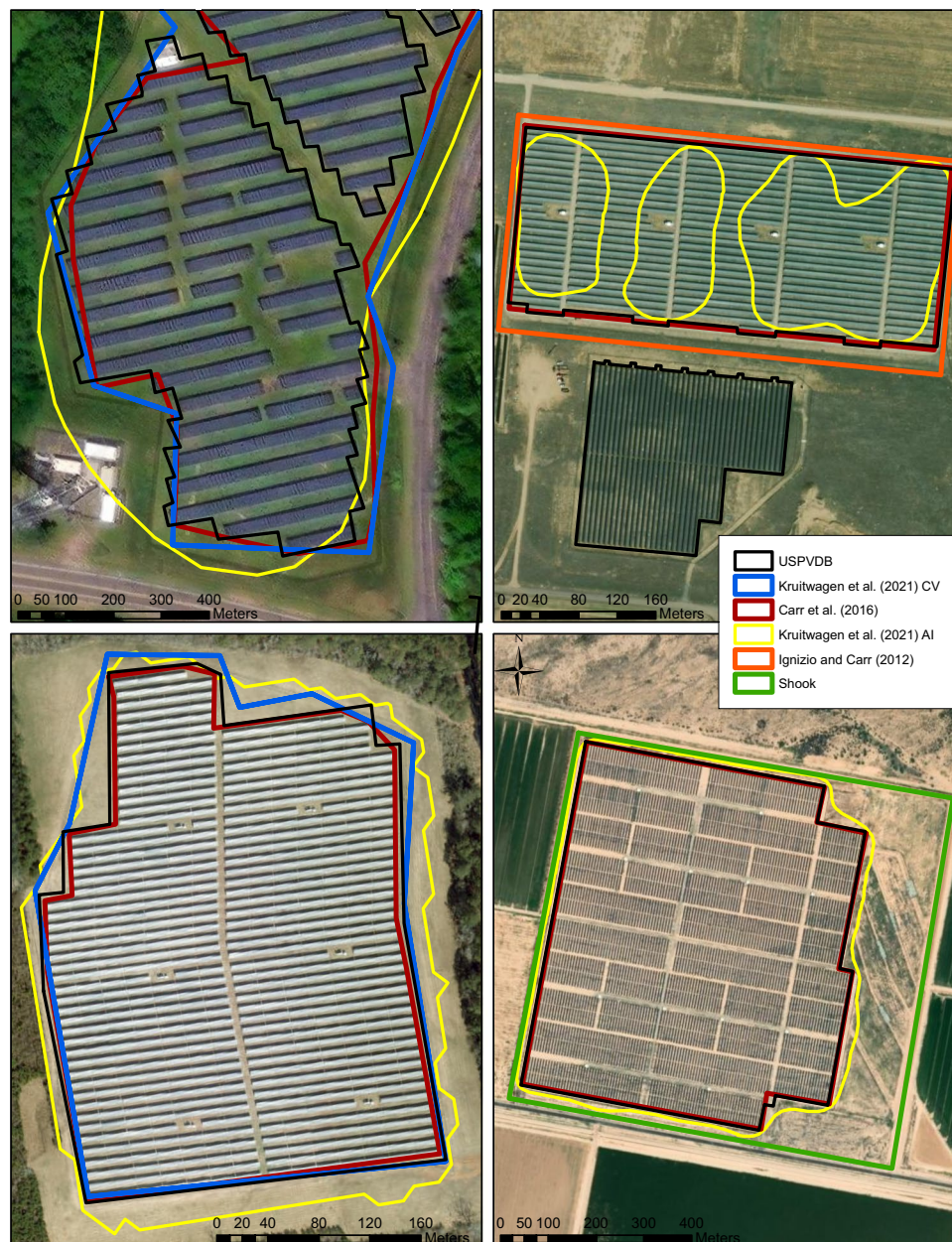
Fig. 5 Polygons generated by different mapping efforts at four PV facilities in the US. Kruitwagen et al. 's polygons were generated by machine learning. Ignizio and Carr, and Shook digitized land transformation, while the other efforts focused on panel area.
