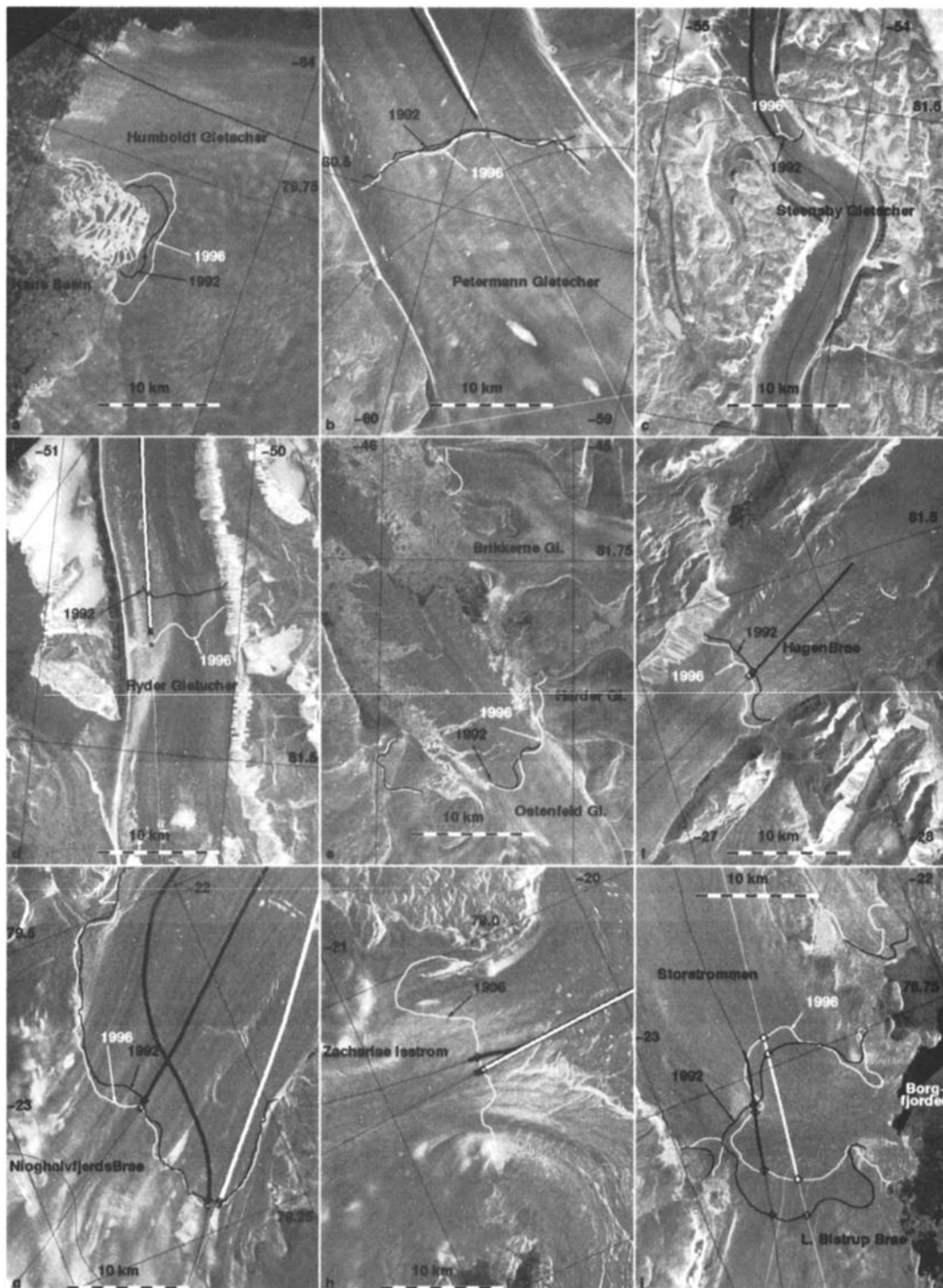
Figure 2. Grounding line migration measured with interferometric SAR (InSAR) between 1992 and 1996 on (a) Humboldt Gletscher, (b) Petermann Gletscher, (c) Steensby Gletscher, (d) Ryder Gletscher, (e) C. H. Ostenfeld Gletscher, (f) Hagen Brae, (g) Nioghalvfjærdsbrae; (h) Zachariae Isstrøm (no 1992 InSAR), and (i) Storstrømmen and L. Bistrup Brae. The location of the grounding line is shown in black for 1992 and in white for 1996, and marked with a pointing arrow. ISR lines are shown in white for 1995 and in solid black for 1999. Intercepts between grounding lines and ISR are marked as diamonds. Bold lines in Figures 2b, 2c, 2d, and 2f-2i denote portions of the ISR track for which ice is in hydrostatic equilibrium, shown in white for 1995 and in black for 1999. Figure 2b includes a 1999 transverse ISR line used to estimate the grounding line ice flux; no ATM elevation was available for that flight because of cloud cover. All plots are overlaid on the radar brightness of the scene from ERS. ERS imagery ©ESA 1996.
