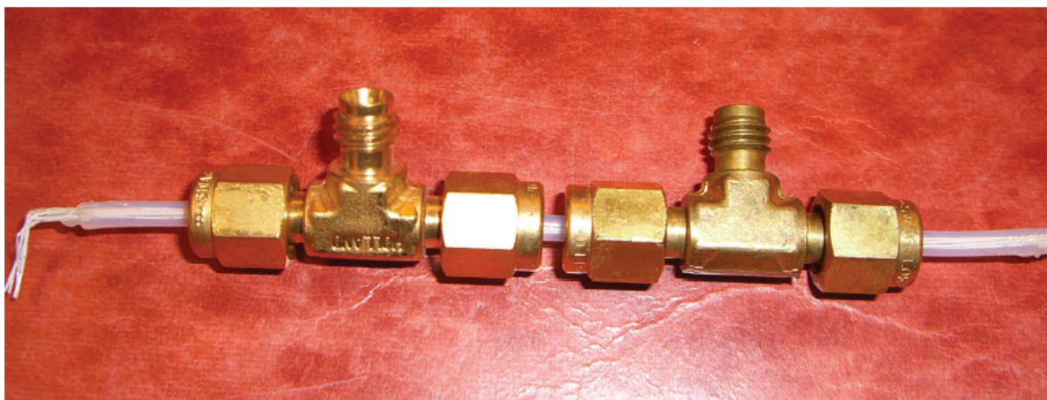
Figure 4.6: Homebuilt Gas Dissolution System. The system consists of bundles of X-50 membrane fibers threaded through 1/8" outer diameter Teflon tubing. The Xe/N 2 /He mixture and water flow in opposite directions, allowing the gas mixture to dissolve into the water by means of a concentration gradient.
