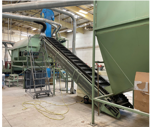
Figure 5.30. Rotary kiln with conveyor and cone tumbler at USDA Forest Service in Placerville.
