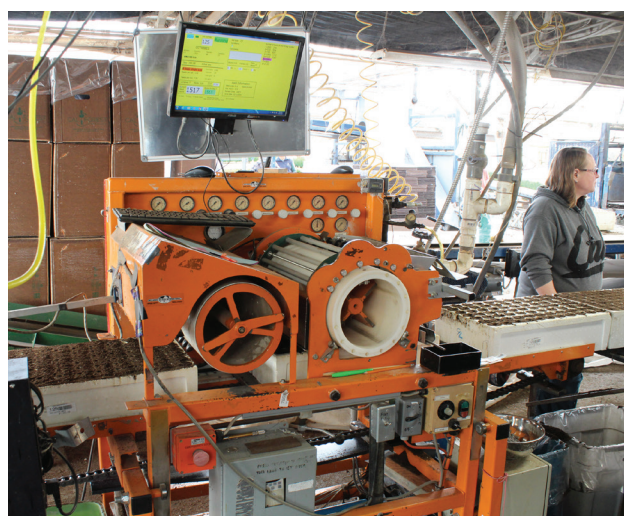
Figure 6.6. A high-speed vacuum seeder sows Styroblocs in a forest nursery. To guide the sowing process, a display above the seeder shows information about the seed lot used.
