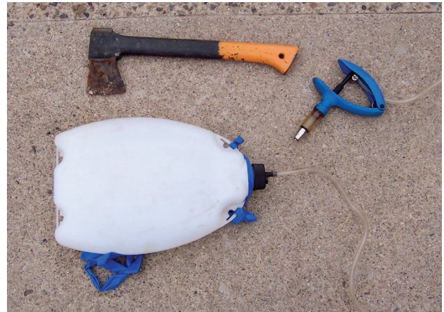
Figure 8.4. Typical forestry hack-and-squirt setup.
