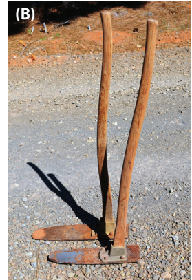
Figure 9.6. When planting flat or relatively gentle slopes, the 100-degree-angled bracket hoe-dad (as shown by the hoedad in the left hand) facilitates setting the blade into the ground at a right angle more easily than the hoedad with a 90-degree-angle bracket, which causes the planter's right hand to contact the ground when setting the blade at a right angle (A). 100-degree-angled bracket in foreground and 90-degree-angled bracket in background (B).
