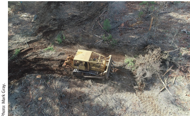
Figure 7.3. Cat with brush rake piling logging slash.
