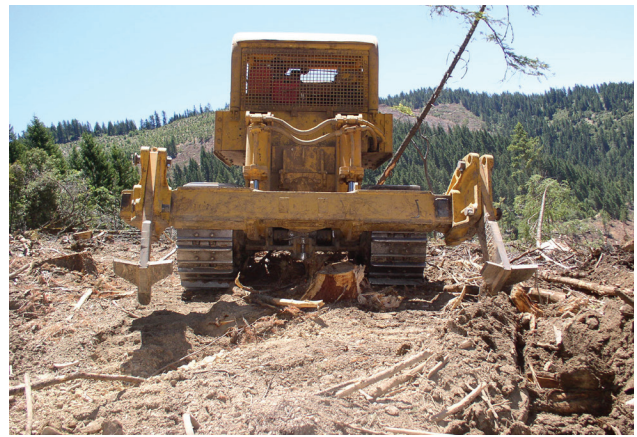
Figure 7.4. D8 Caterpillar with winged subsoiler shanks.
