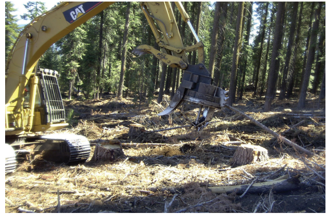
Figure 7.8. VH mulcher mounted on an excavator.
