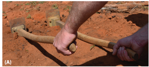
Figure 9.6. When planting flat or relatively gentle slopes, the 100-degree-angled bracket hoe-dad (as shown by the hoedad in the left hand) facilitates setting the blade into the ground at a right angle more easily than the hoedad with a 90-degree-angle bracket, which causes the planter's right hand to contact the ground when setting the blade at a right angle (A). 100-degree-angled bracket in foreground and 90-degree-angled bracket in background (B).
