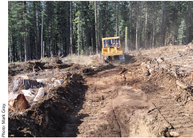
Figure 7.7. V-blade clearing landing slash for planting.
