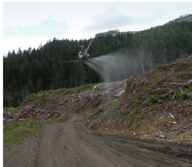
Figure 8.2. Example of a split-boom application.
