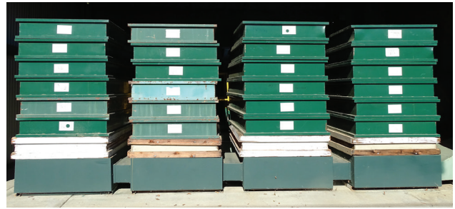
Figure 5.29. Batch kiln with kiln boxes loaded onto plenums for cone drying at Lewis A. Moran Reforestation Center in Davis.
