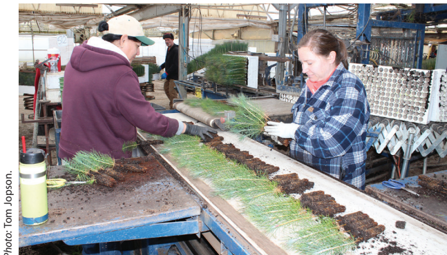
Figure 6.7. A containerized seedling extraction, grading, and packing line.
