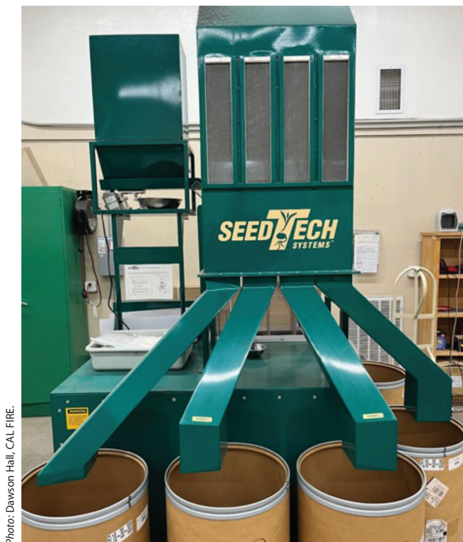
Figure 5.35. Four-chamber forced-air separator (free-standing).
