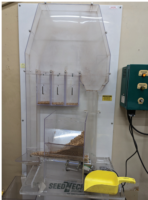
Figure 5.34. Wall-mounted pneumatic separator (vacuum version).
