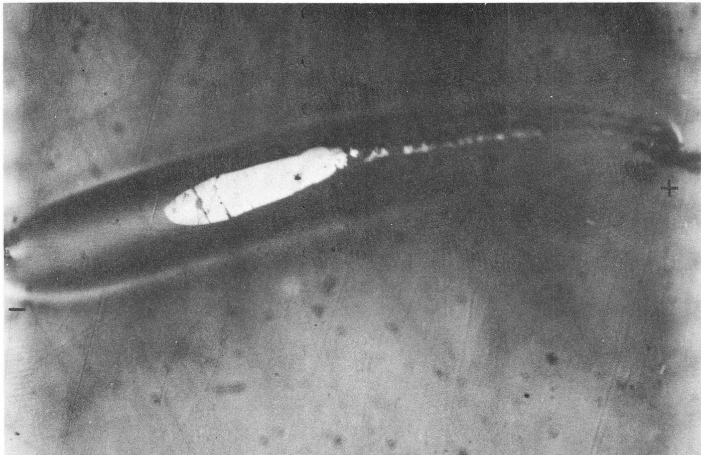
Fig. 10. A subsurface filament which has changed to the "leaf" structure during growth 1000 \times , unetched.
