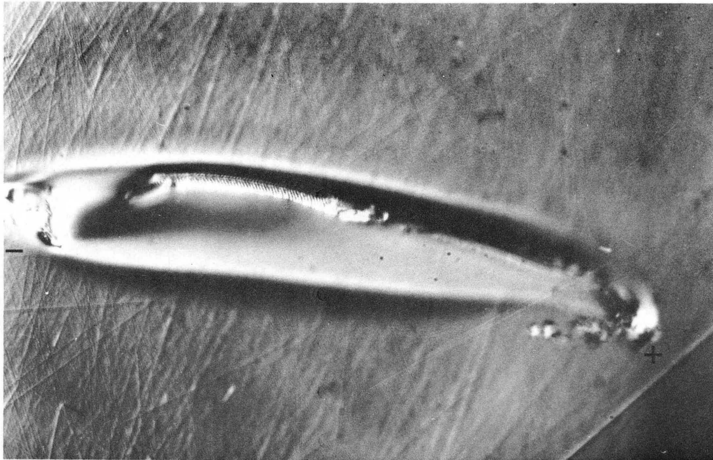
Fig. 8. A filament with initial and final subsurface growth, showing blocky second phase growth at the negative probe 1000 \times , unetched.
