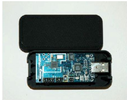
Figure 1: A Tmote Sky, by Moteiv, shown in a custom enclosure.
